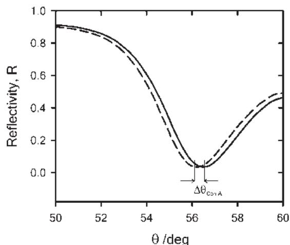
**Figure 4.** Reflected intensity as a function of the angle-of-incidence scan ( $\theta$ ) for a mannosylated Au electrode before (dashed line) and after (solid line) Con A binding ( $1 \mu\text{M}$ , pH 7.4).  $\Delta\theta$  is proportional to the mass of native Con A immobilized on the electrode surface.
