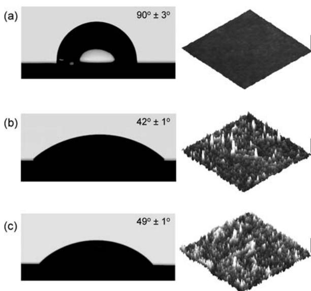
**Fig. 5** Atomic force imaging and contact angle measurements corresponding to: (a) alkyne-functionalized Si surface, (b) PSSNa- $\text{N}_3$ -modified Si surface and (c) PMETAC- $\text{N}_3$ -modified Si surface.
