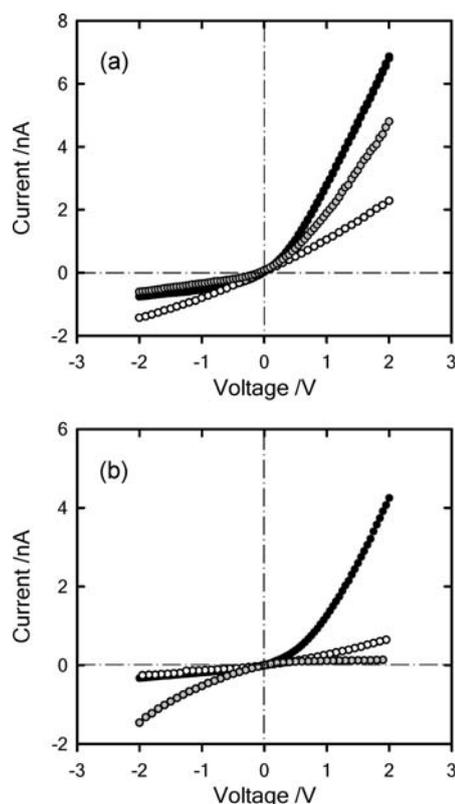
**Fig. 8** Current–voltage curves corresponding to nanochannels in 0.1 M KCl modified with: (a) PSSNa- $\text{N}_3$  having tip diameter  $d = 8$  nm and (b) PMETAC- $\text{N}_3$  having tip diameter  $d = 5$  nm. The different colours indicate: (black) carboxylated nanochannel, (white) alkyne-modified nanochannel and (gray) polyelectrolyte-modified nanochannel.
