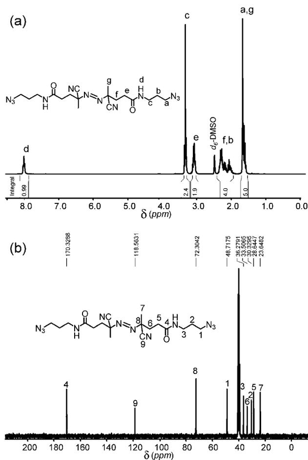
**Fig. 1** (a)  $^1\text{H-NMR}$  (b)  $^{13}\text{C-NMR}$  spectra in  $d_6$ -DMSO of the azide-terminated azo initiator.
