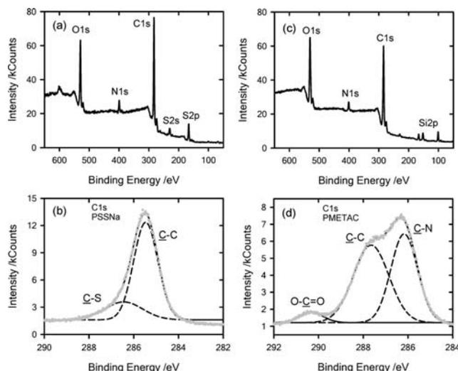
**Fig. 6** XPS analysis corresponding to: (a) PSSNa-modified silicon, broad spectrum, (b) PSSNa-modified silicon, 1Cs region, (c) PMETAC-modified silicon, broad spectrum, (d) PMETAC-modified silicon, C1s region.
