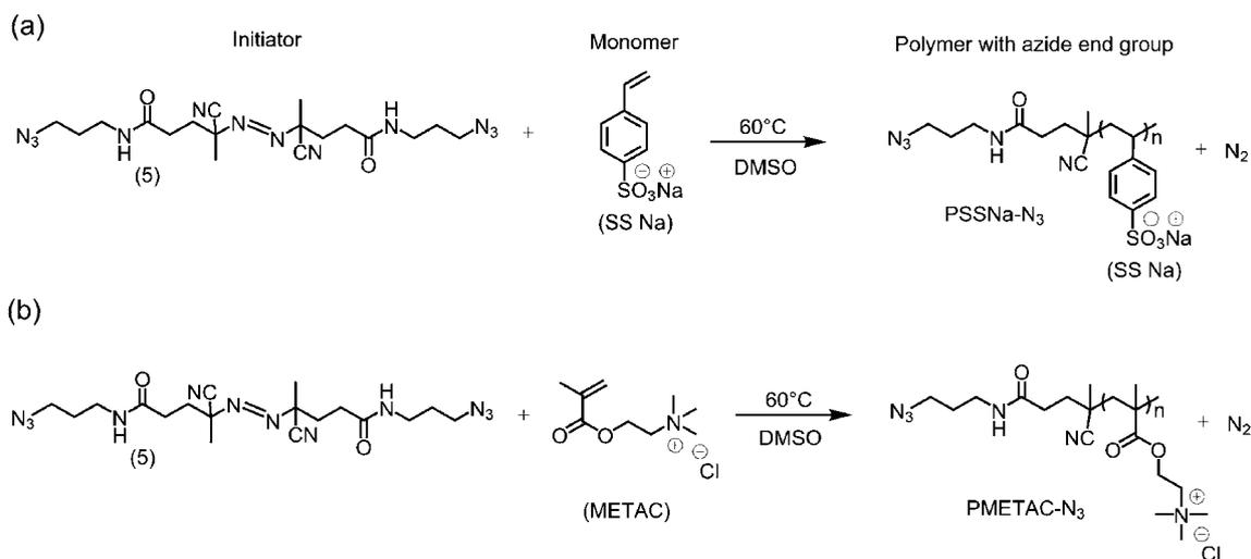
**Scheme 2** Scheme describing the polymerization of (a) azide-terminated sodium polystyrene sulfonate (PSSNa– $\text{N}_3$ ) and (b) azide-terminated poly(2-methacryloyloxyethyl-trimethylammonium chloride) (PMETAC– $\text{N}_3$ ).
