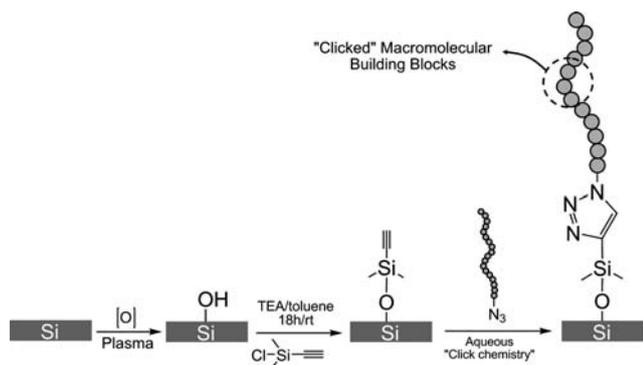
**Fig. 4** Scheme describing the functionalization of the silicon surface with alkyne groups followed by the “clicking” of the polyelectrolyte chains.
