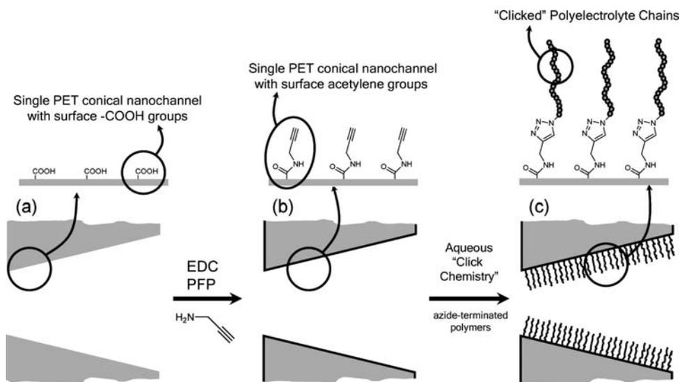
**Fig. 7** A scheme showing the surface chemical modification of the COOH-functionalized PET conical nanochannels (a) with alkyne groups (b) followed by the “clicking” of the polyelectrolyte chains (c).
