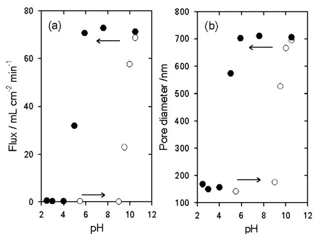
**Fig. 10** Changes in flux (a) and pore diameter (b) as a function of pH. The filled and open circles represent data generated after a pH 10.5 pretreatment and after a pH 2.5 pretreatment, respectively. Reproduced and adapted with permission from Lee *et al.*, *J. Am. Chem. Soc.* 2006, **128**, 8521. Copyright 2006 American Chemical Society.
