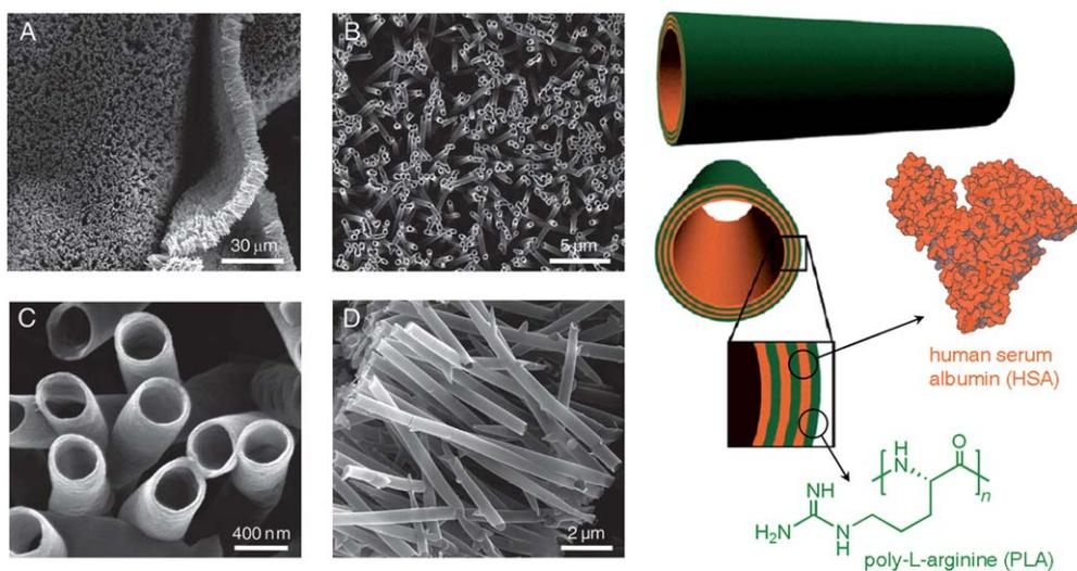
**Fig. 11** Scanning electron microscopy images at different magnifications (A–D) of (PLA/HSA)<sub>3</sub> nanotubes prepared using polycarbonate track-etched nanomembranes. The figure also includes a descriptive cartoon showing the constituting building blocks of the multilayer assembly. Reproduced and adapted with permission from Qu *et al.*, *ACS Nano* 2010, **4**, 563. Copyright 2010 American Chemical Society.
