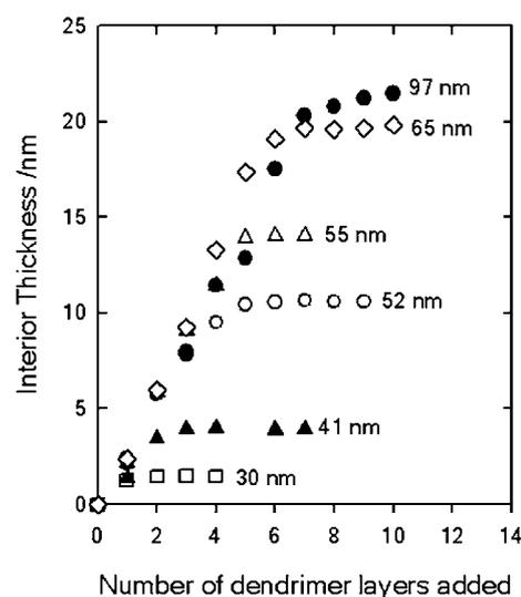
**Fig. 4** Thicknesses of the dendrimer polyelectrolyte layers deposited in the interior of the AAO nanomembranes from 100 mM NaCl aqueous solutions, as determined by optical waveguide spectroscopy (OWS). The data labels indicate the initial membrane pore diameters. In comparison, the dendrimer diameter is 7 nm. Reproduced and adapted with permission from Lazzara *et al.*, *ACS Nano*, 2010, 4, 3909. Copyright 2010 American Chemical Society.
