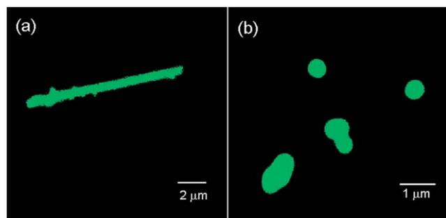
**Fig. 7** Confocal laser scanning microscopy images of LbL-grown nanotubes (a) and the resulting nanocapsules (b) constituted of (PSS/PAH)<sub>6</sub>PAH assemblies after hydrothermal treatment at 121 °C. Images were taken in water and PAH was labeled with fluorescein isothiocyanate to facilitate the visualization of the nanostructures. Reproduced and adapted with permission from He *et al.*, *Langmuir*, 2008, **24**, 5508. Copyright 2008 American Chemical Society.
