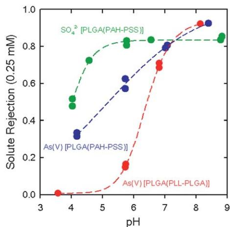
**Fig. 9** Effect of solution pH on the ion separation of 0.25 mM As(V) (Na<sub>2</sub>HAsO<sub>4</sub>) or Na<sub>2</sub>SO<sub>4</sub> solutions using polycarbonate track-etched nanomembranes modified with PLGA-based assemblies. Reproduced and adapted with permission from Hollman *et al.*, *Langmuir* 2004, **20**, 5418. Copyright 2004 American Chemical Society.
