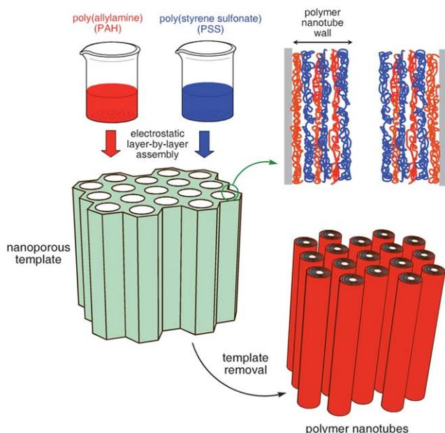
**Fig. 1** Simplified representation of the formation of polyelectrolyte nanotubes through sequential assembly of polycations and polyanions inside the nanoporous template and the subsequent removal of the nanotemplate.
