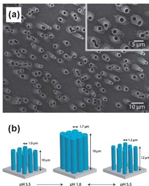
**Fig. 8** (a) SEM images of substrate-attached LbL-grown (PAH/PAA) nanotube arrays. (b) Schematic illustration describing the dimensional changes of the tube arrays immersed in solutions with different pH conditions. Reproduced and adapted with permission from Chia *et al.*, *Langmuir* 2009, **25**, 14044. Copyright 2009 American Chemical Society.
