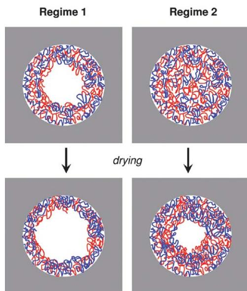
**Fig. 5** Schematic representation of the structural organization of polyelectrolyte multilayers in nanopores according to the scenario proposed of Jonas and co-workers. The cartoons describe both regimes prior to and after drying. Reproduced with permission from Roy *et al.*, *Langmuir*, 2010, **26**, 3350. Copyright 2010 American Chemical Society.
