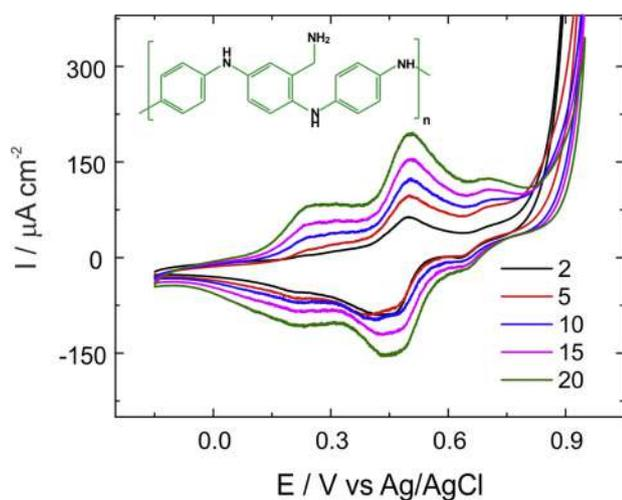
**Fig. 1.** Cyclic voltammograms of the PABA electropolymerization for different cycle numbers, indicated in the plot.  $v = 50 \text{ mV s}^{-1}$ .
