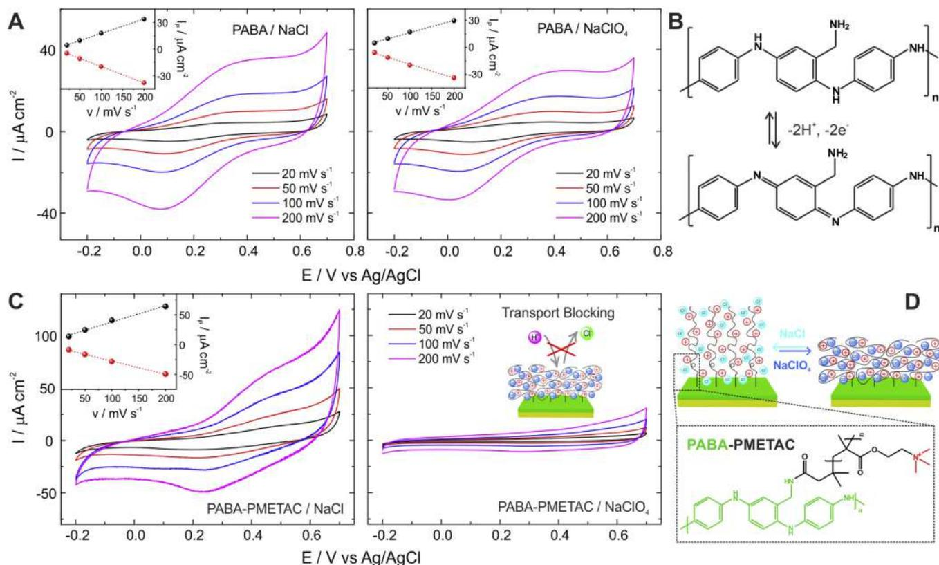
**Fig. 5.** (A) Cyclic voltammetry of PABA modified electrodes in NaCl solution (left) and NaClO<sub>4</sub> (right). (B) Redox process occurring at PABA. (C) Cyclic voltammetry of PABA-PMETAC modified electrodes in NaCl solution (left) and NaClO<sub>4</sub> (right). (D) Schematic representation of the conformational changes that occurs at PABA-PMETAC modified electrodes. Insets in panels A and C show the dependence of the current peak on the sweep rate.
