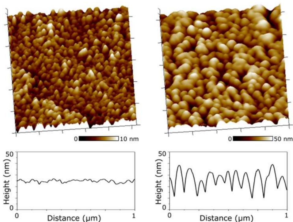
**Fig. 3.** AFM topography images and height profiles corresponding to PABA-modified Au substrates before (left) and after (right) the PMETAC brush-grafting. Note the scale differences in the height of the images.
