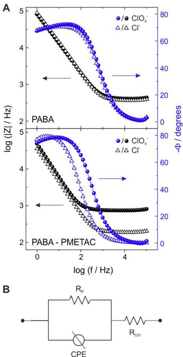
**Fig. 6.** (A) Bode plots for PABA and PABA-PMETAC modified electrodes ( $E = 0.4$  V). Circles correspond to  $\text{NaClO}_4$  and triangles to  $\text{NaCl}$  solutions. (B) Equivalent circuit used for fitting the EIS results.
